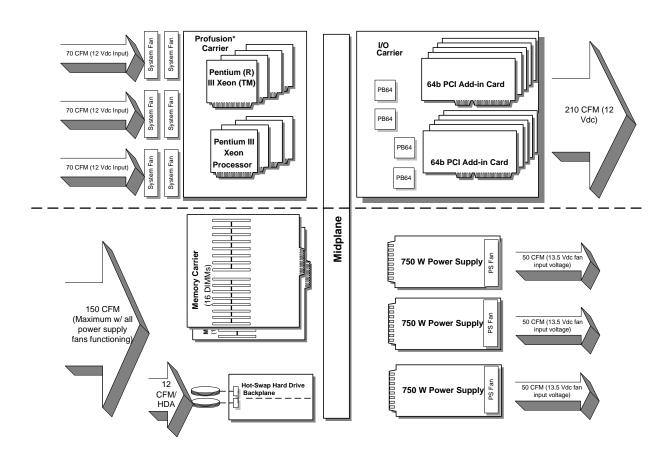
Figure 3-8: OCPRF100 MP Server System Cooling
